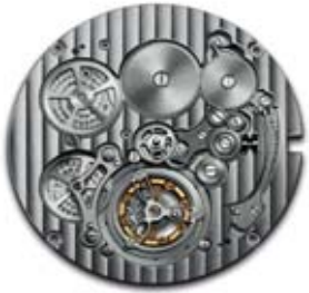
FINISSIMO BVL 268 CALIBER EXTRA-THIN FLYING TOURBILLON Mechanical manufacture movement with manual winding. Extra-thin flying tourbillon, thickness of 1.95 mm. BVL 268 caliber decorated by hand with côtes de Genève and anglage finishing. Power reserve around 52 hours.
